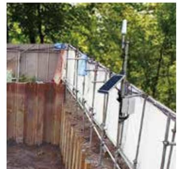
Measurement of displacement of landslide prevention walls
