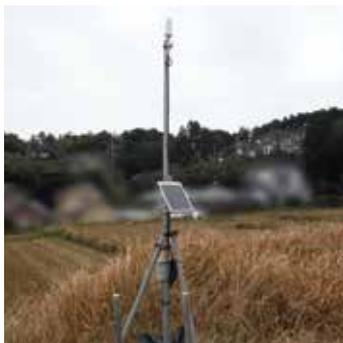
Measurement of ground surface displacement above tunnels
