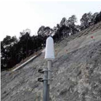
Embankment slope displacement measurement
